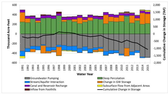
On **Figure 20**, positive numbers indicate inflows into the Subbasin aquifer, while negative numbers indicate outflows from the Subbasin aquifer.
