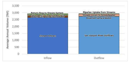
The land surface water budget for the Projected Conditions Baseline is shown on **Table 5-3** and has average annual supplies of 900,000 AFY. Supplies are comprised of precipitation (270,000 AFY), applied surface water (293,000 AFY), applied groundwater (315,000 AFY), and riparian uptake from streams (22,000 AFY). Demands total 898,000 AFY and are comprised of evapotranspiration (536,000 AFY), surface runoff and return flow (134,000 AFY) to the stream system, and deep percolation (228,000 AFY).
