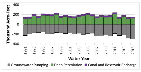
Figure 5-11: Groundwater Recharge and Extraction – Modesto Zone
