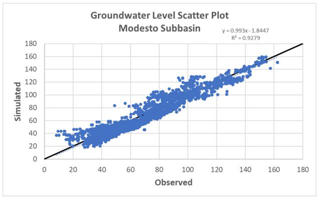
Figure 30: Modesto Subbasin Simulated vs. Observed Scatter Plot
