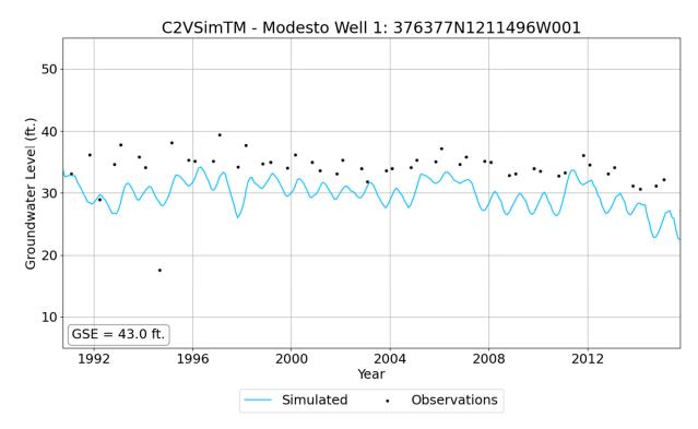
Figure 16: Modesto Calibration Well 1, Simulated and Observed
