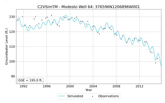
Figure 22: Modesto Calibration Well 64, Simulated and Observed
