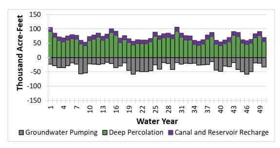
Figure 5-33: Projected Conditions Groundwater Recharge and Extraction – Oakdale South Zone
